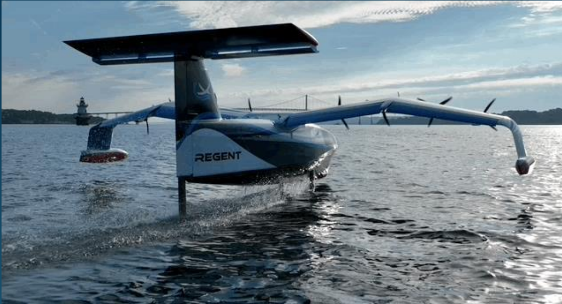
Wave tolerance demonstration of hydrofoils on REGENT's 1/4 scale seaglider prototype
